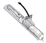
• Pull the paper lower side from the camera head in the direction of the handpiece.
