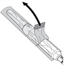
Pull off the paper underside from the camera head in the direction of the handpiece.
