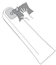
With the interchangeable head removed, clean the surface of the image sensor using the cleaning set for VistaCam Optik.
